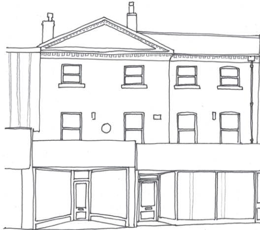
EXISTING UNSYMPATHETIC SHOP FRONT THAT DOES NOT TAKE ACCOUNT OF THE HOST BUILDING
