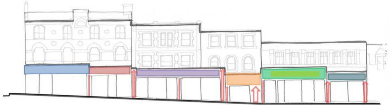
LOSS OF RHYTHM: FASCIA'S THAT CONTINUE OVER SEVERAL BUILDINGS OR SPLIT A BUILDING IN TWO BREAK UP THE RHYTHM OF THE STREET. OVERSIZED GLAZING AND FASCIA'S CREATE A HORIZONTAL EMPHASIS.
